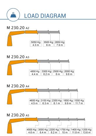
Only for use with hook - sea state 0 or harbour condition. For other uses or conditions, contact us." When operating with winch, loads must be reduced by the weight of installed winch
