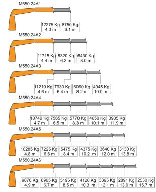
Only for use with hook - sea state 0 or harbour condition. For other uses or conditions, contact us." When operating with winch, loads must be reduced by the weight of installed winch
